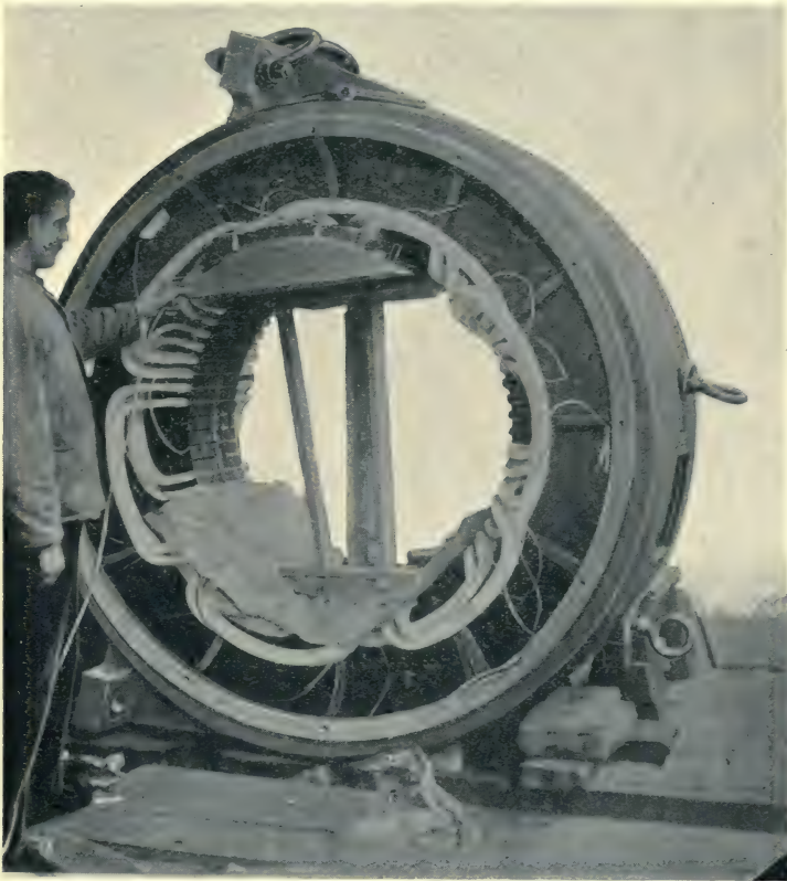
FIG. 372.—Winding Three-phase, Whole-coiled, Double-coil Winding in Three Ranges (Two Ranges completed)—(Bruce Peebles).
